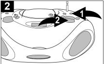
To repeat all of the tracks on a disc continuously, press the REPEAT/FM MONO button **①** twice while in the Stop mode; " *□*" will appear in the display. Press the PLAY/PAUSE (▶II)/MEM-UP button **②** to begin playback.
